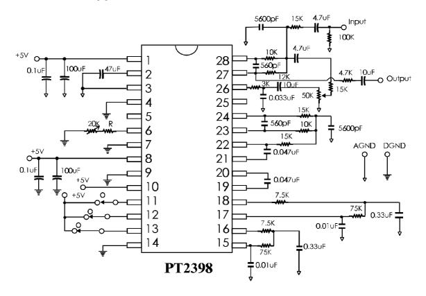
Note: External Resistor having a value of 10 K Ohms to 50 K Ohms may be used. The recommended Resistor Value (R) is 10 K Ohms. When the value of the Resistor (R) increases, the range of the Delay Time also increases.
